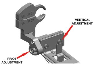
STEP 4 - When the mount is positioned as far forrward as it will go, tighten the clamp screw untill the Top and Mid Sections are slightly snug around the mirror stem. You should still be able to rotate the mount. Rotate the mount so it is parallel with the bottom of the mirror. Tighten the clamp screw untill the mount is securely attached to the mirror stem.
